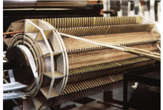
Ventilated Dry-Type Transformer Coil. Both SG-200 and FHT Laminates are used in a wide variety of dry-type transformer
